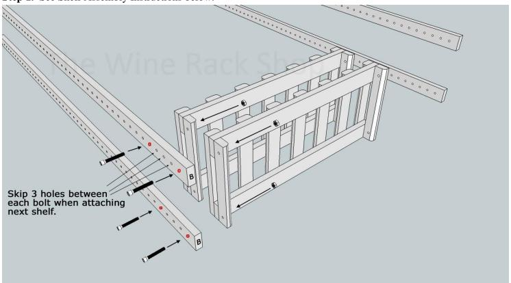
**Step 2.** Shorter bolts connect shelf to rack uprights on **end of racks**. Racks connect together using **longer bolts** which pass through a shelf, a common upright, and shelf on opposite side of rack upright. See below.
