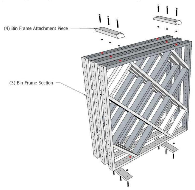
**Step 2.** Rack uprights marked with "B" on ends will be at bottom of rack and will sit on Baseboard Assembly. Attach rack uprights to Bin Frame Sections with nuts and bolts. Use highlighted holes in rack uprights and highlighted holes in Bin Frame Sections. Tighten bolts with Allen Wrench provided.
