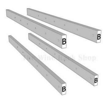
**Step 2.** Insert bolt through pre-drilled lowest(1<sup>st</sup>) rack upright hole and pre-drilled shelf hole. Hand-tighten nut on inside of shelf. Repeat this for each of the four shelf holes and all four rack uprights.
