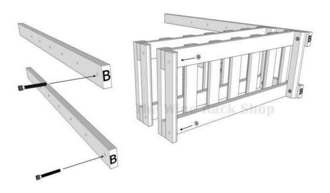
**Step 3.** After all shelves are fastened with bolt and nut stand rack on rack uprights ends marked with "B". Use Allen wrench and tighten bolts completely. Bolt heads should sink slightly into wood rack upright. Slide entire rack onto baseboard unit. Slide rack top over rack uprights and onto rack.
